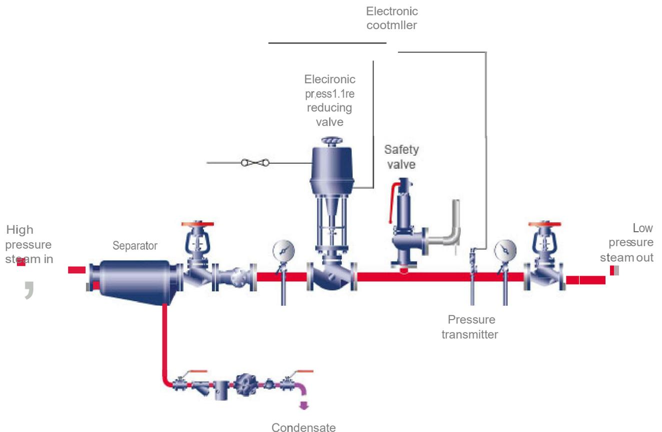
FIGURE 1 GENERAL ARRANGEMENT OF AN ELECTRIC PRESSURE REDUCING STATION
